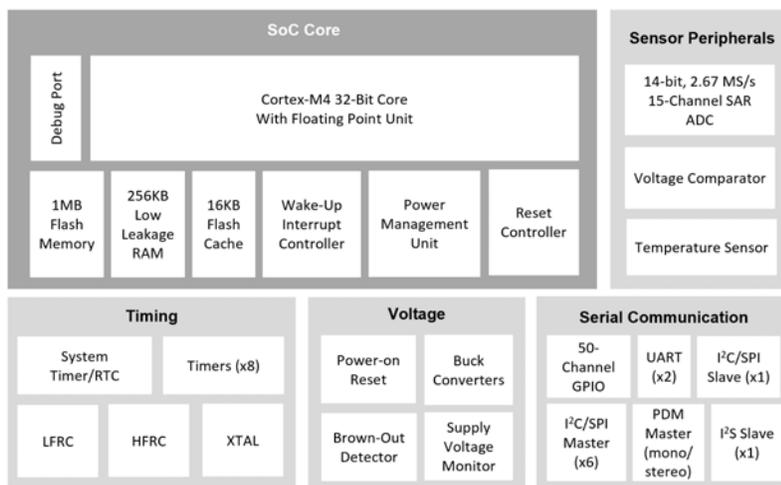
Block Diagram for the Ultra-Low Power Apollo2 Thin SoC
