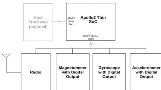
Typical Sensor Application Circuit for the Apollo2 Thin SoC
